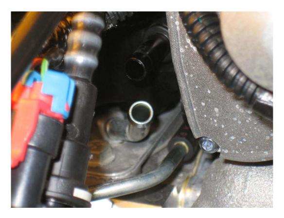
As you can see above, the silver port that goes into the valley cover is the PCV "source" for the catch can, and the black port above it is the "return" to the throttle body from the catch can.
