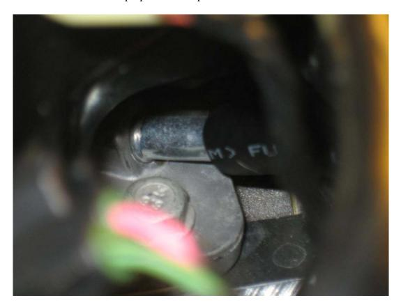
Next I cut the hose to the proper length to the fitting on the catch Can. This connection goes to the top brass Catch Can barb. I then placed one of the supplied hose clamps onto the end of the hose (you can use a pair of pliers to squeeze the two prongs on the clamp to open it), and push the hose onto the top hose barb as seen here.
