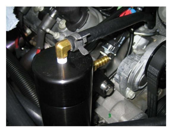
Once that was completed, I installed the remaining hose onto the return port on the back of the throttle body. This port is colored black and it also does not require a hose clamp. Here is a picture of the port and then with the hose mounted to it.
